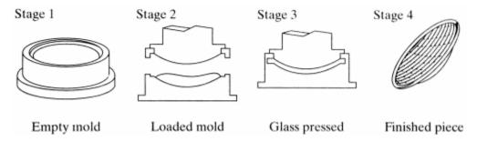
Figure 4. Molding of lenses [source: Kalpakjian & Schmid]
