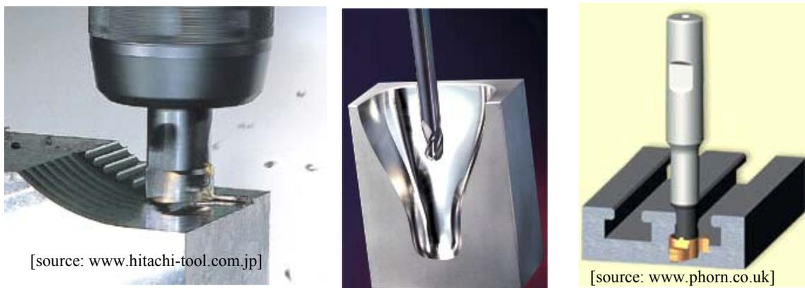
Figure 15. End milling (a) A Flat end mill being used to cut a curved surface (b) Ball end mill used for finish-cuts on a mold (c) Formed end-mill: here, a T-slot cutter is shown cutting a T-slot
