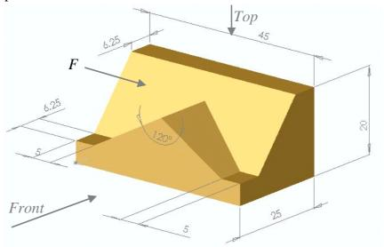
(ii) Using the orthographic views, make a projection view that shows the face marked F in true size. This view must show all faces that are visible in the TOP view of the part.
