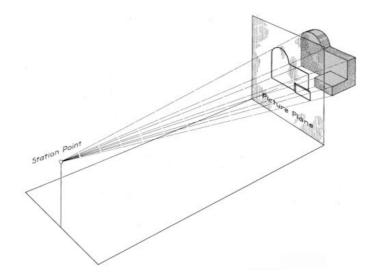
(1) If any face that is completely behind the picture plane will appear in true size, then every line on this face must appear in true size.
