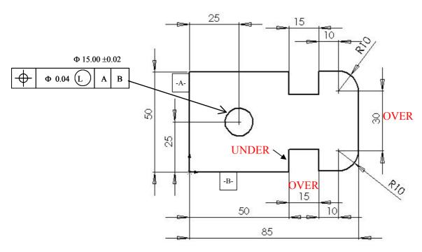
(i) Among the dimensions on the drawing, identify and mark one example of overdimensioning, and one example of under-dimensioning. Give reason for your answer (one line max, for each case).
