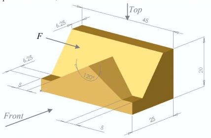
(ii) Using the orthographic views, make a projection view that shows the face marked  $\mathbf{F}$  in true size. This view must show all faces that are visible in the TOP view of the part.
