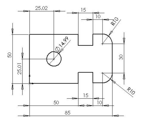
Limits on hole size are [14.98, 15.02], so the size of the hole in the above part is OK.
