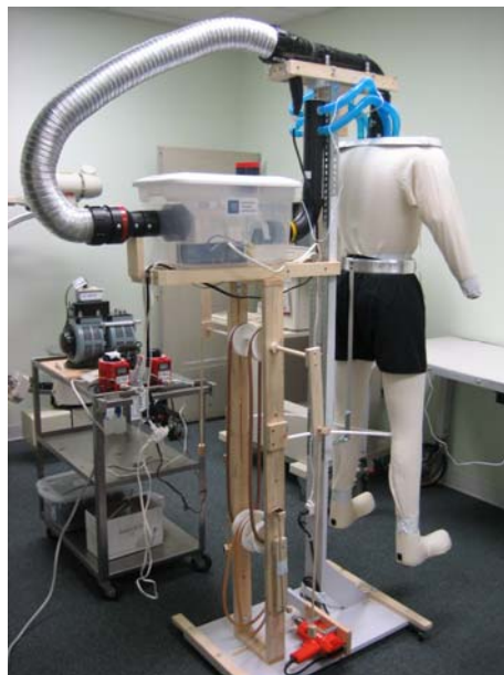
Figure 2. Inflatable thermal manikin used for assessing the effectiveness of the prototype vests. The photograph illustrates a semi-nude (control) manikin configuration
