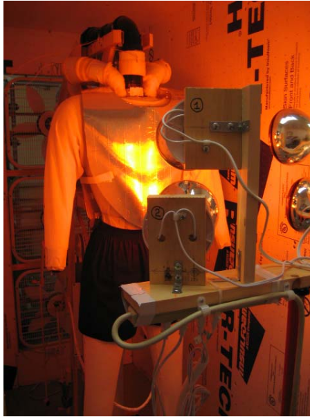
Figure 3. Illustration of inflatable thermal manikin exposed to infrared heat radiation while wearing prototype vest. The heat radiation produced by the four IR lamps was directed onto the chest of the manikin.
