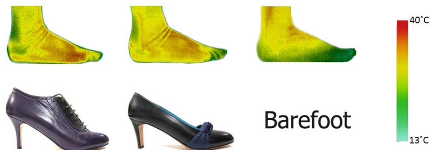
Figure 1. Thermal images after wearing two types of footwear for one hour
