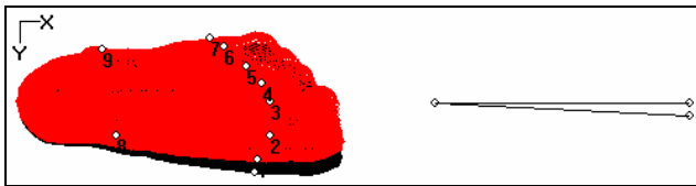
Fig. 3. Foot alignment method based on the pternion and a landmark on the second metatarsal (landmark 3)
